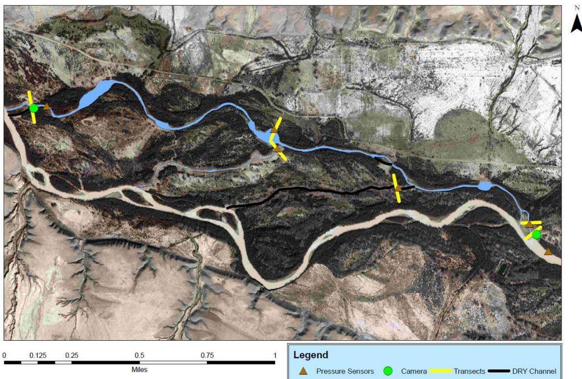
**Figure 1. Phase II restoration site with the approximate location of channel cross-sections, pressure sensors, and field cameras.**
