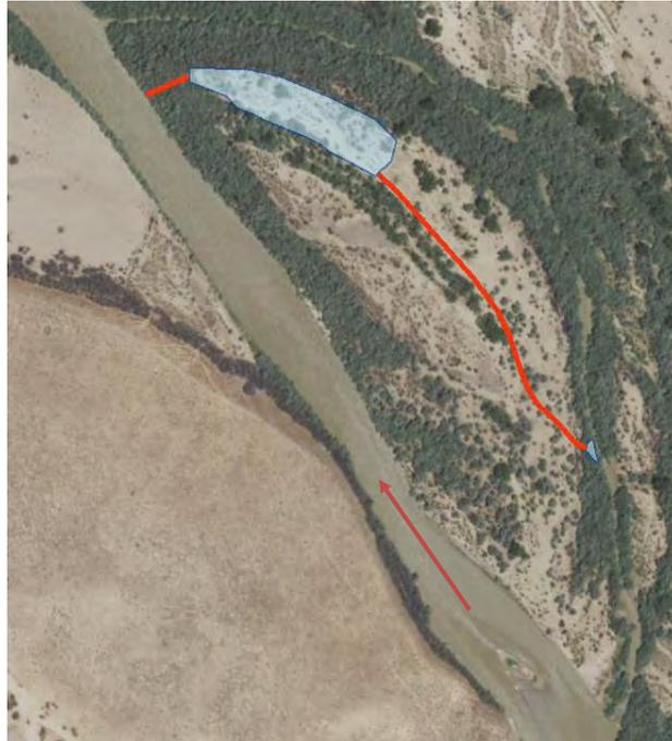
Figure 2. Aerial photograph and Keller-Bliesner's wetland design concept at San Juan River mile 107 (Appendix I). The red arrow depicts direction of river flow. The large blue polygon is the wetland and the smaller one is the stilling basin at the inlet from the secondary channel. The other red lines represent channels for water transfer into and out of the wetland.
