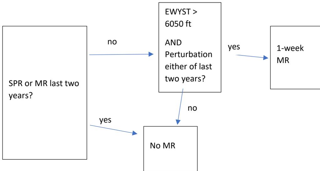
V1.6 This simplistic rule fires MRs in any year that an SPR is not triggered, so long as the EWYST is above 6018 ft. If it doesn't put the reservoir into a shortage in that year, it triggers a release.
