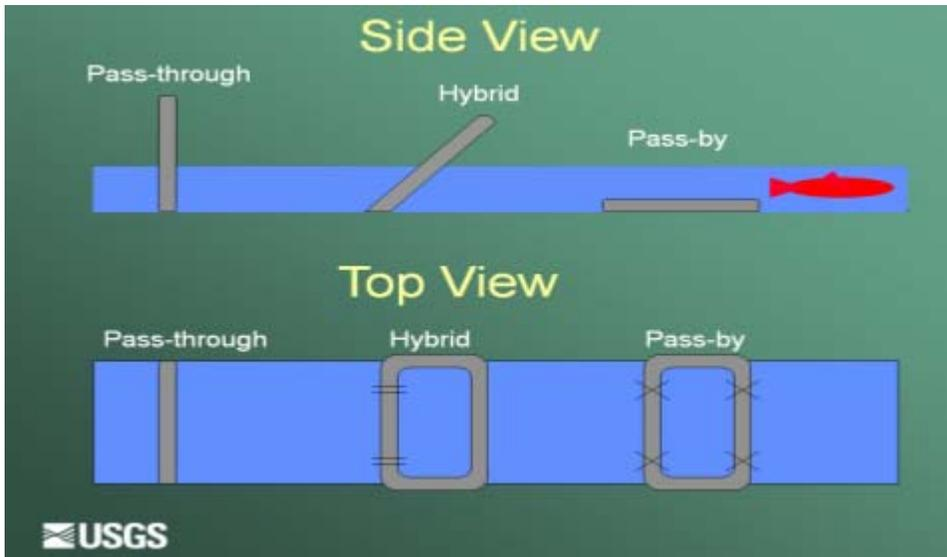
Figure 5. Different methods for securing the antenna loops. Note hybrid method for the proposed Maybell Ditch system.
