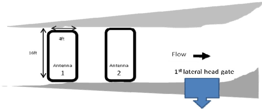
Figure 3. Schematic (not to scale) of proposed PIT detection system for the Maybell Ditch. Antenna 2 is located immediately downstream of antenna 1 (ca. several feet) but upstream of all lateral irrigation head gates.
