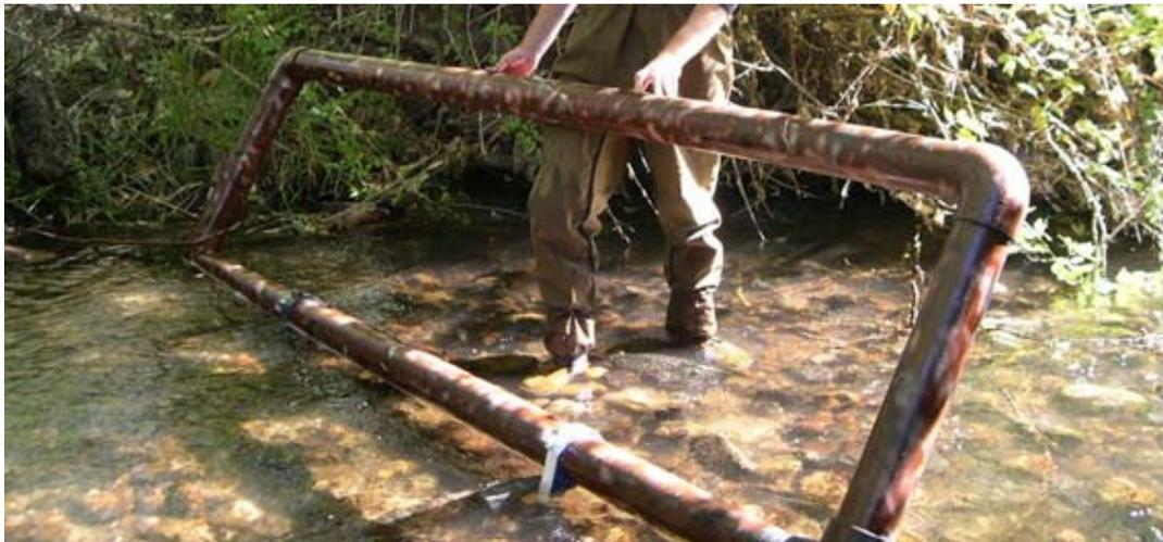
Figure 4. Antenna loop secured on the bottom of the loop to function as a hybrid pass through/pass by antenna.
