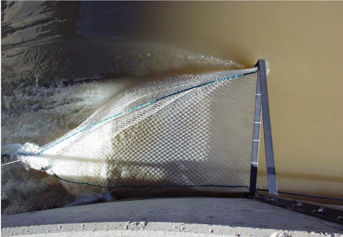
**Figure 7. View from above spillway net.**
