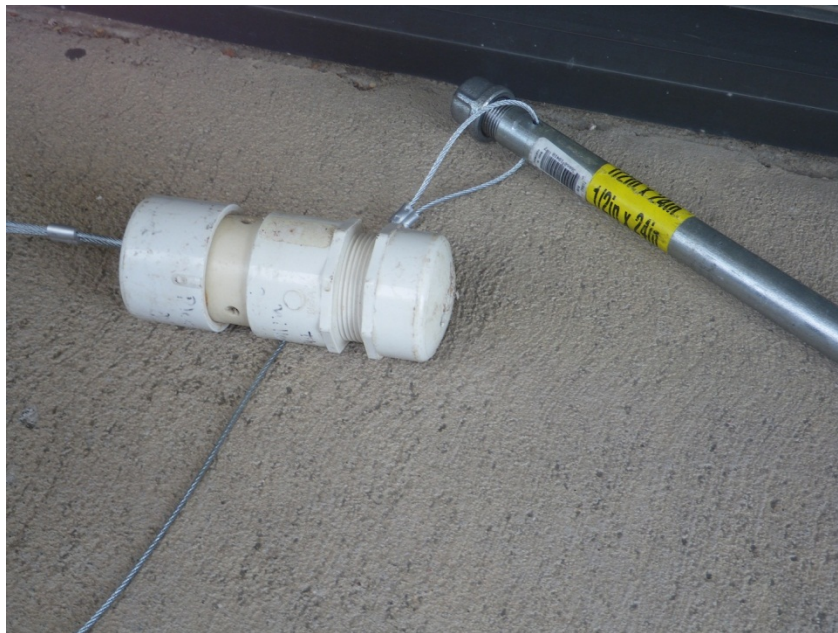
Figure 2. Example data logger housing, closed and ready for deployment.
